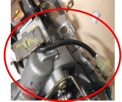
Step 1 – There are two black wires going out of the controller box. One goes directly to the ECU connector / plug. The other one, you must connect it to a +12 Volt ignition switched supply. Attention – this black wire must be connected to an ignition switched supply and not a permanent supply.
